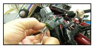
**3.** Locate the blue seal pins in unused ports #16 & #32. Remove the seal pin plugs from #16 & #32 (push out from terminal side with pick). Insert the terminated green wire into pin 32, and the white wire into pin 16 on the "wire side" of the connector.
