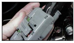
**7.** You can now position the Pigtail cable for easy access to your computer cable. Use the provided rubber dust cap to protect the open end of the mini USB Pigtail while not in use.
